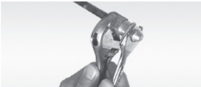
Figure 8 Carefully support the nozzle adapter when removing or installing nozzle
