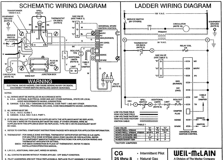
10. CIRCULATOR IS FIELD INSTALLED AND WIRED FOR PFG-5 BOILER.
