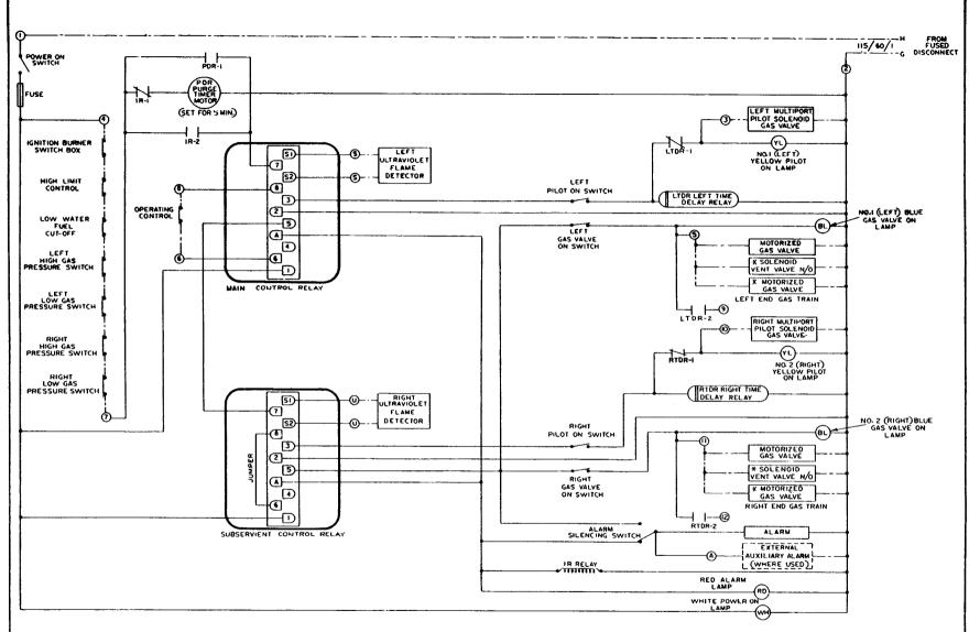
FIELD WIRING ----**FACTORY WIRING -**CONTROL RELAY TERMINAL (4) CONTROL PANEL TERMINAL \*Not required for factory mutual specifications.
