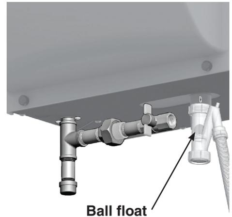
**⚠WARNING** Contact a boiler service technician immediately if you find the trap dry (no water inside).
