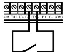
**NOTE:** On a sensor fault while the Enable/Disable terminals are open, the control will follow the Enable /Disable state regardless of the sensor fault condition.
