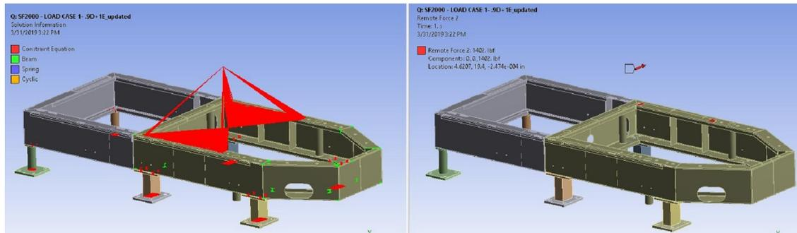
Figure 1- Loads acting on the boiler structure
