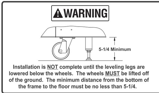
5. Extend mounting legs further as needed until the boiler is level. Check level, front to back as well as side to side. Measure level on top panel of boiler NOT across the heat exchanger, since it is intentionally tilted within the boiler enclosure.
