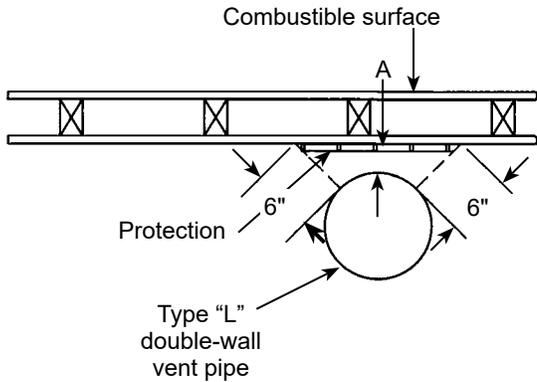
**Figure 28** Back vent clearances
