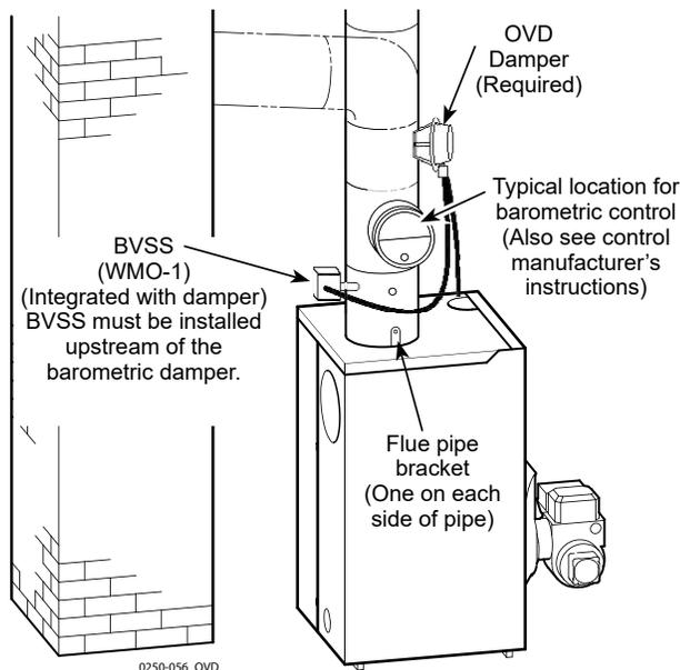
**Figure 10** Top outlet breeching connection for models which do not require a vent damper.
