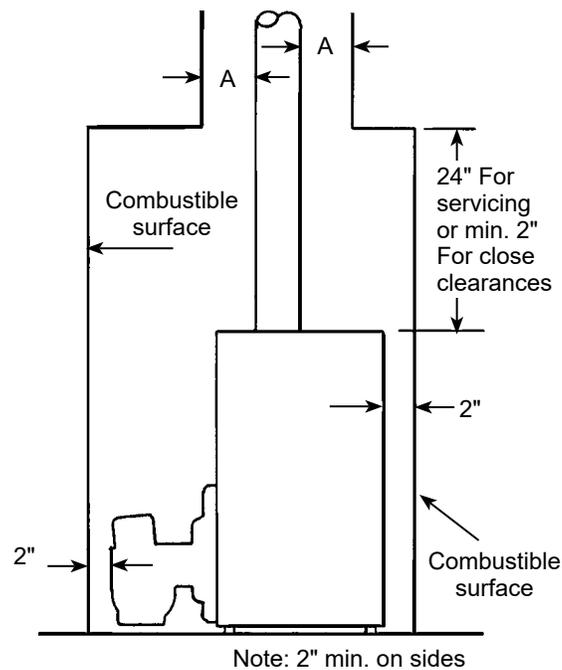
\* All clearances measured from outer surface of equipment to combustibile surface, not to the protection used.
