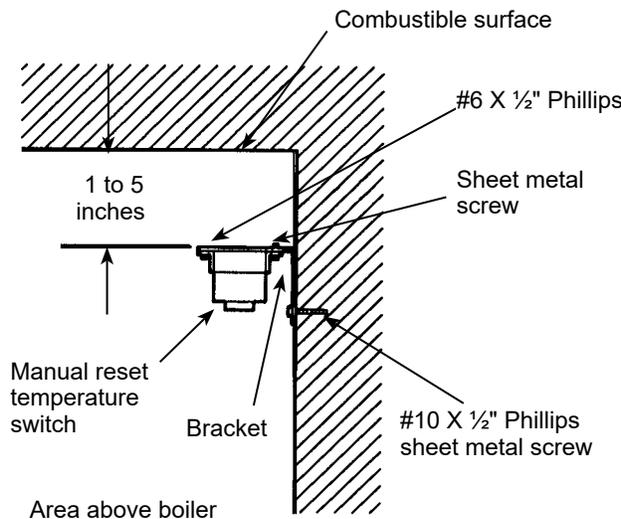
**Figure 26** Manual reset temperature switch wiring
