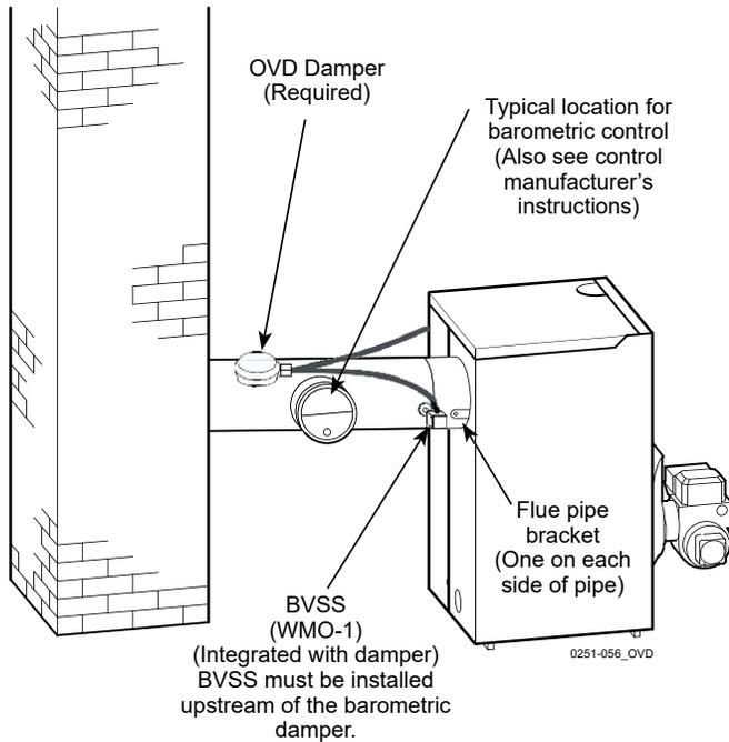
**Figure 9** Back outlet breeching connection for models which do not require a vent damper.
