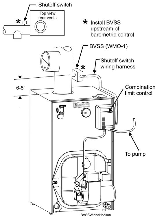
**Figure 21** BVSS wiring diagram
