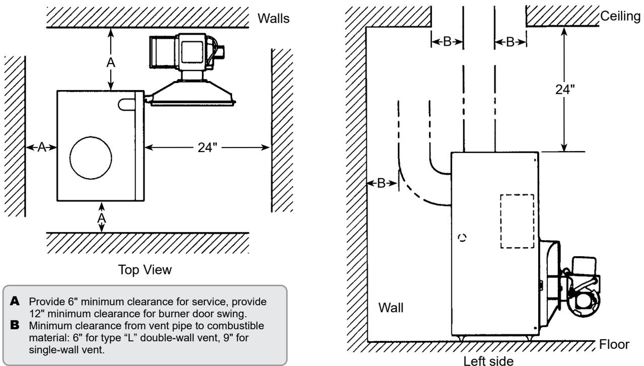
**A** Provide 6" minimum clearance for service, provide 12" minimum clearance for burner door swing.
