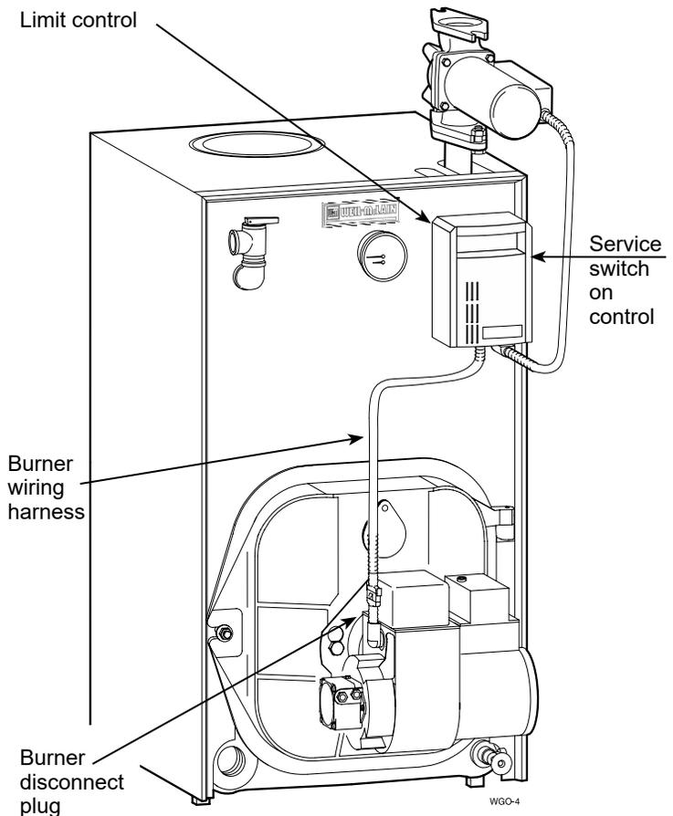
**THE LIMIT CONTROL SUPPLIED WITH THE BOILER MUST BE SET-UP WITH THERMAL PREPURGE OR THERMAL TARGETING ACTIVE UNLESS EXEMPTED BELOW:**
