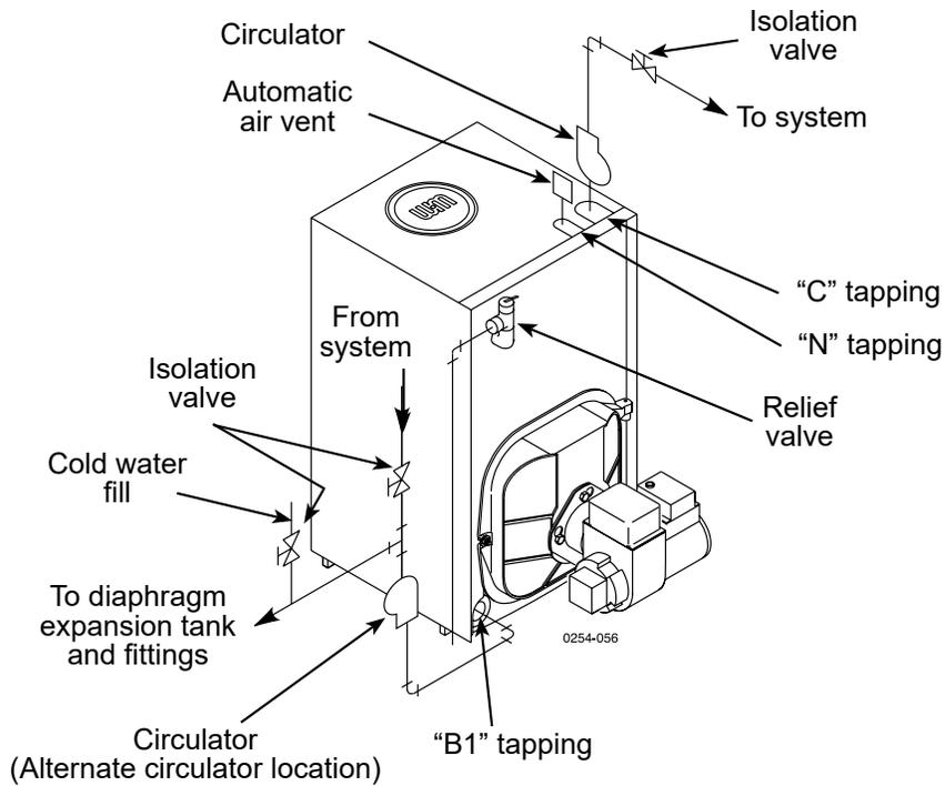
**Figure 12** Piping with CLOSED expansion tank
