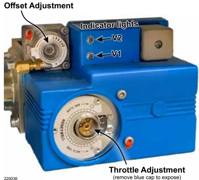
Figure 71 Throttle and offset regulating screws
