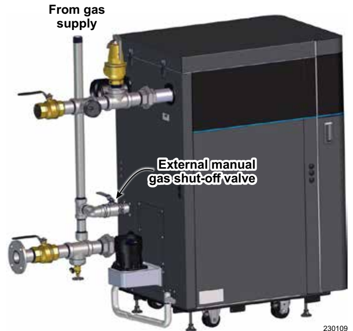
Figure 53 Gas supply piping connection (fittings and gas valve supplied by installer)
