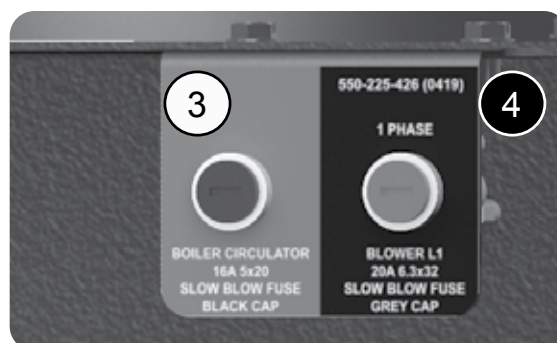
Figure 99 SVF 2500/3000 Circulator and blower fuse location
