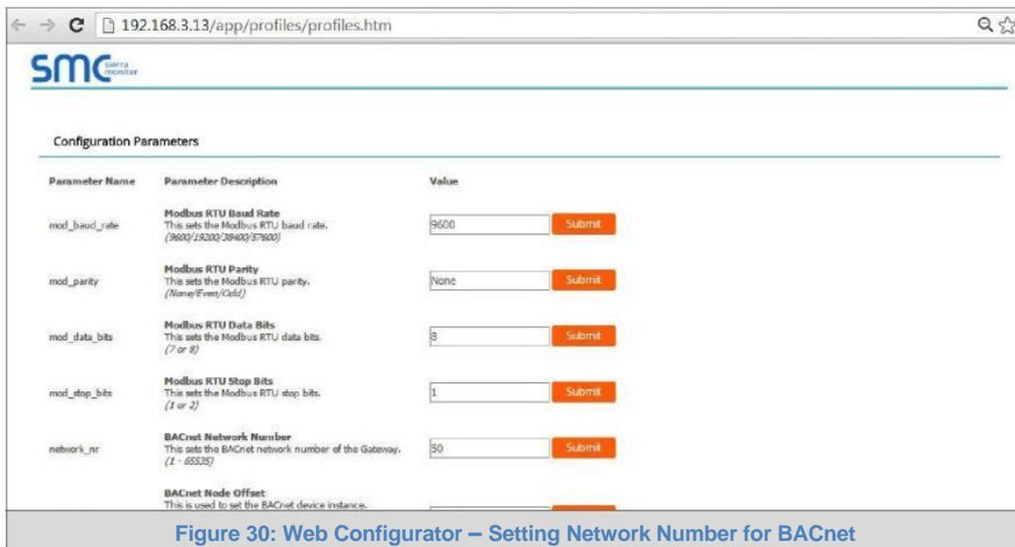
Figure 30: Web Configurator – Setting Network Number for BACnet
