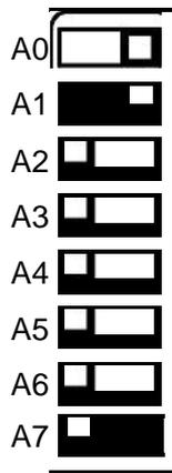
Figure 7: MAC Address DIP Switches
