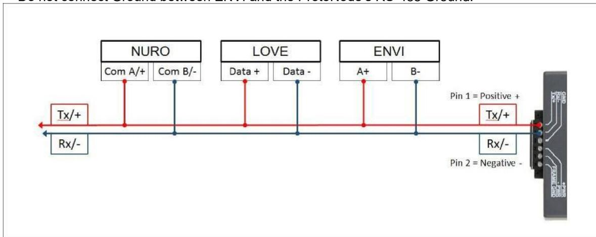
Figure 11: Wiring diagram for Modbus RTU RS-485 connections to the ProtoNode's RS-485 port
