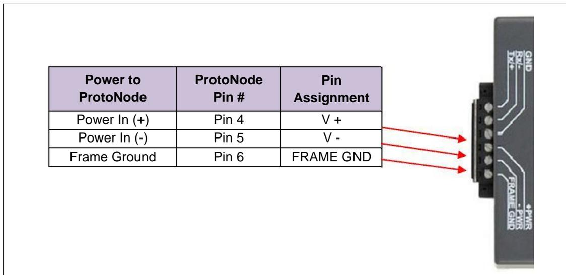
**Figure 18: Power Connections**
