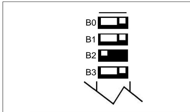
Figure 8: BMS Baud Rate DIP Switches
