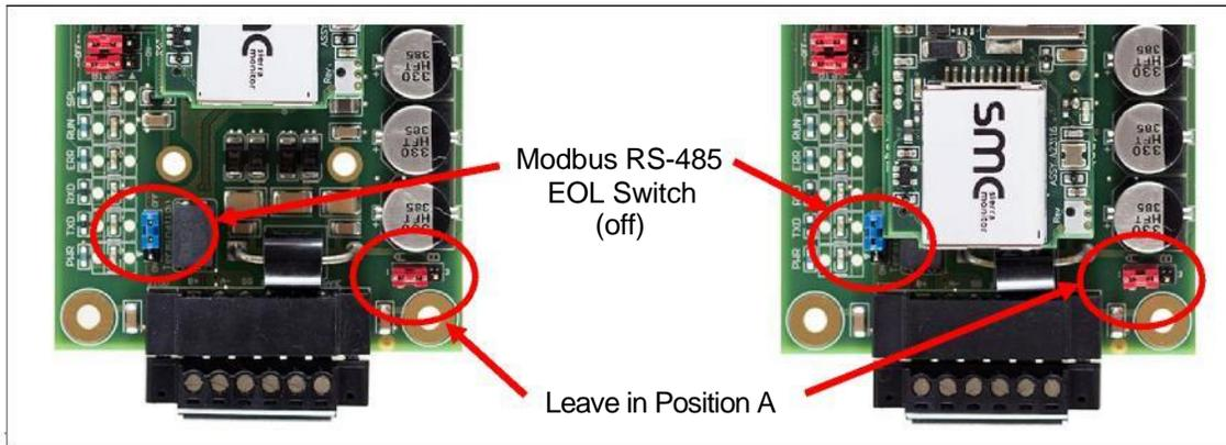
Figure 13: Modbus RS-485 End-Of-Line Termination Switch on the ProtoNode N34 (left) and ProtoNode N35 (right)
