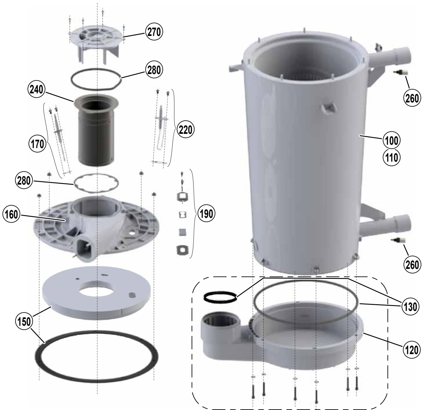
Figure 137 Heat exchanger assembly - Evergreen ® Pro 299/300/399 (see Figure 136, page 178 for part numbers)
