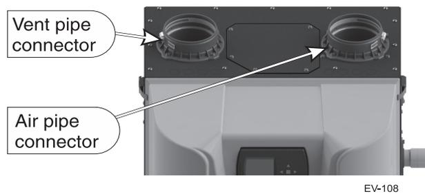
**WARNING ADAPTERS** — Use adapters if using other than 4-inch PVC or CPVC. This is required for different materials or if using 3-inch pipe.
