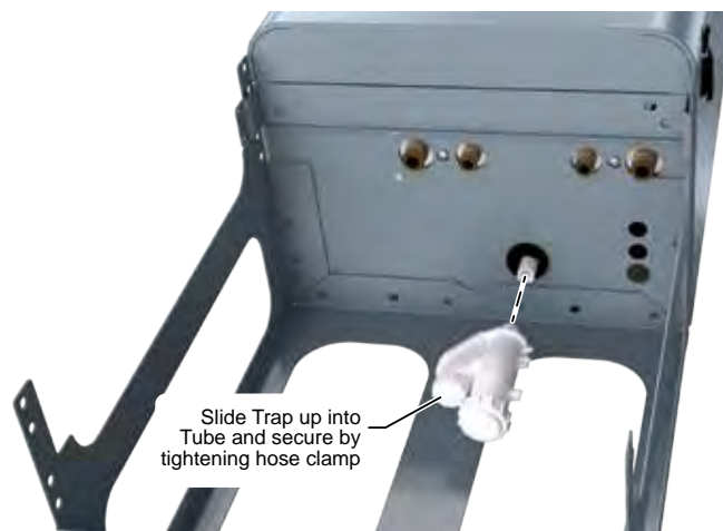
Figure 73 Condensate outlet tube and condensate trap connection (front access panel removed)
