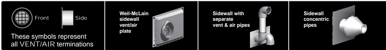
Figure 32 The vent termination must be located to meet all requirements below (also applies to vertical vent terminations). The minimum distance from adjacent public walkways, adjacent buildings, open able windows and building in the National Fuel Gas Code, ANSI Z223.1/NFPA 54 and/or the Natural Gas and Propane Installation Code, CAN/CSA B149.1. The vent termination clearances below are for U.S.A., for Canadian vent termination clearances please refer to the requirements of CAN/CSA B149.1 Natural Gas and Propane Installation Code. Consideration should be given to avoid possible damage caused by vent plumes and condensate when choosing a venting configuration and location. Maintain a minimum clearance of 4 ft. (1.22m) horizontally from, and in no case above or below, unless a 4 ft. (1.22m) horizontal distance is maintained, from electrical meters, gas meters, regulators, and relief equipment.
