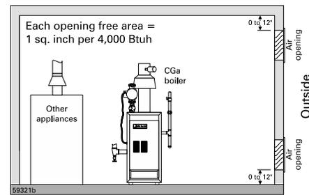
**Figure 4** Air from outdoors — vertical ducts
