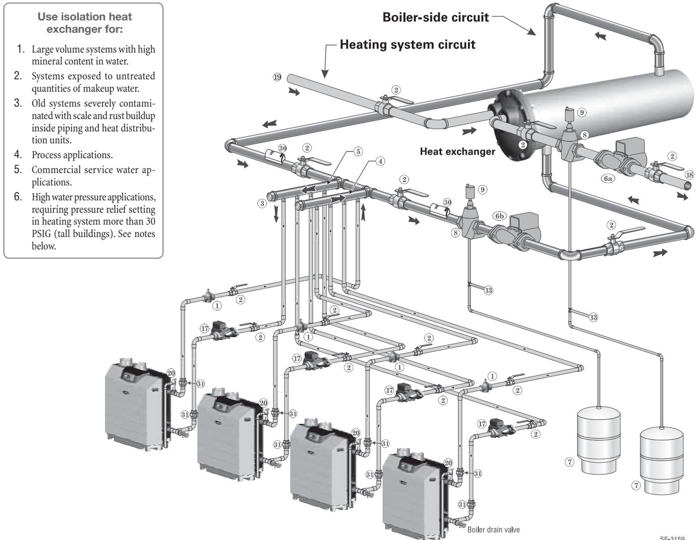
**NOTICE** **Heat exchanger type** — This illustration shows a shell and tube exchanger. Other exchanger types may be used if suitable for the system water conditions.
