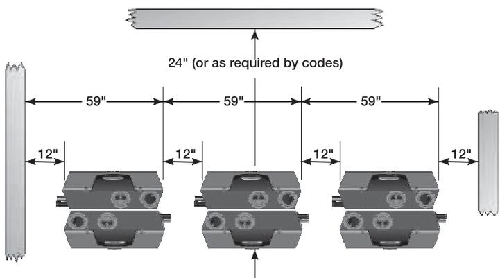
**Figure 5** Manifolded combustion air option
