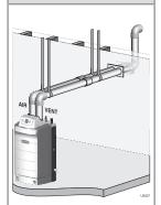
Sidewall termination with separate vent and air pipes (Go to page 39)
