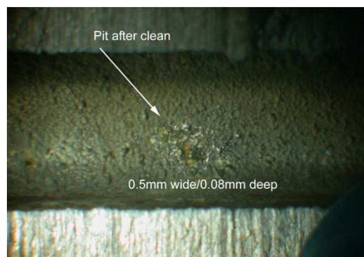
**#6 Corrosion checking after cleaning of the aluminum HE water way in a hard water system**
