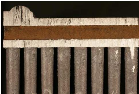
**#3 Cross section of an Aluminum HE water way from a soft water system**
