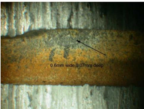
**#5 Corrosion checking after cleaning of the aluminum HE water way in a soft water system**
