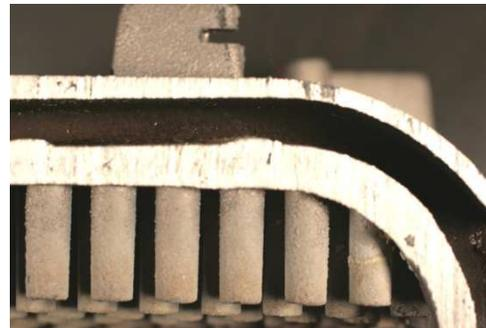
**#4 Cross section of an Aluminum HE water way from a hard water system**
