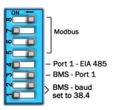
5. Connect the communications wiring to Port 1a. Connect to **Net+**, **Net-**, and **Gnd**.
