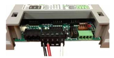
2. The UPC must be connected to the BAS via Port 1A. Use provided three pin connector. See below.
