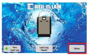
2. Select the < Display Setup > to enter the setup for COM Ports and Gateway
