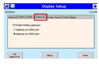
**NOTICE** Do **Not** enable "Gateway" on COM1, this will cause errors.
