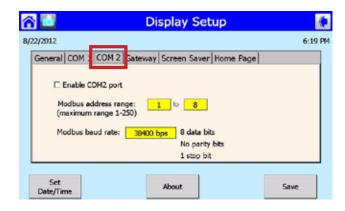
Ensure the Modbus baud rate matches the gate way requirements.
