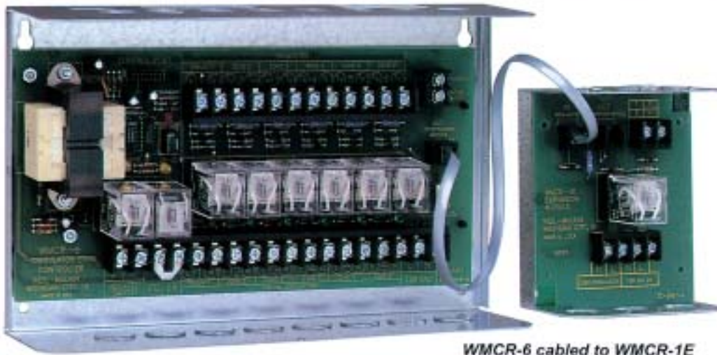
WMCR-6 cabled to WMCR-1E
