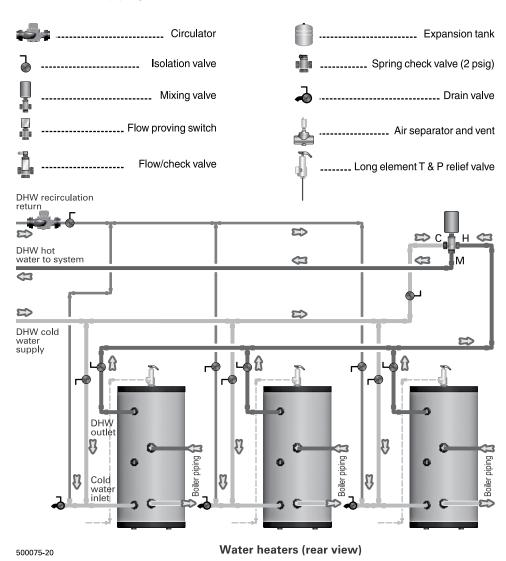
Figure 13 Alternate methods of revers-return piping and Easy-Fit® Manifold detail
