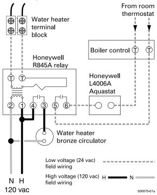
Install the Honeywell L4006A aquastat in the boiler, below the water line. Set for a temperature of 180 to 190°F to control boiler temperature when there is no call for steam heating.
