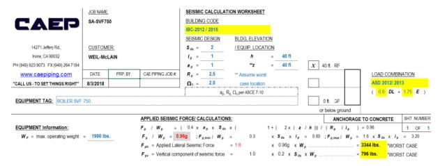
2- Load calculation for LRFD (used in the analyses of the anchorage)
