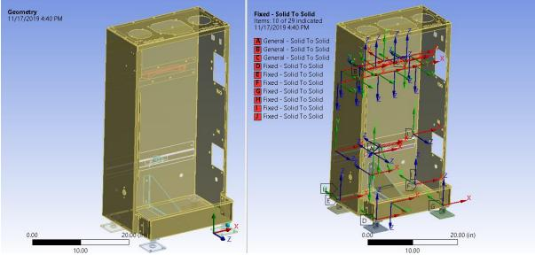
Figure 2- FE model of the boiler and joint/contact definitions
