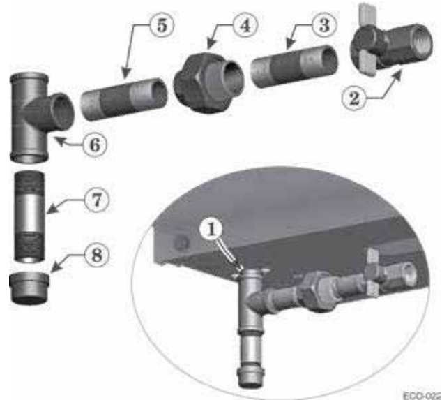
Figure 67 Connect gas supply piping
