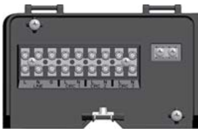
Figure 80 Field wiring overview (see Figure 83, page 72 and Figure 84, page 73 for detailed schematic and ladder wiring diagrams) (top view shown at bottom right is of WM97+70/100 — electrical entrances for WM97+155 are the same)
