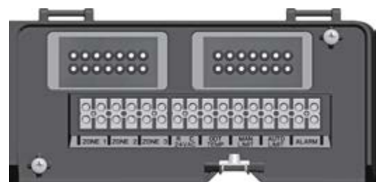
Figure 80 Field wiring overview (see Figure 83, page 72 and Figure 84, page 73 for detailed schematic and ladder wiring diagrams) (top view shown at bottom right is of WM97+70/100 — electrical entrances for WM97+155 are the same)
