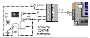
Wiring the control to GV90+ (1135-700), CGa (1135-05/606), CGi (1135-615), and the EG Water (1135-605) boiler controls
