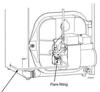
See local codes for appropriate arrangement and piping of filter control valves, etc., back to oil tank.
