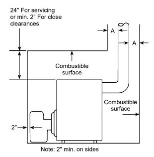
Figure 29 Top vent clearances
