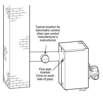
**Figure 8** Top Outlet Breeching for models which require a vent damper.
