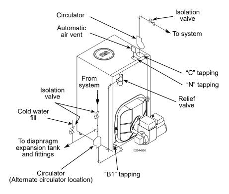
Figure 12 Piping with CLOSED expansion tank
