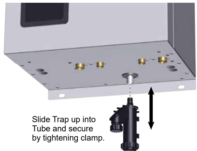
Figure 64 Condensate outlet tube and condensate trap connection (front access panel removed)
