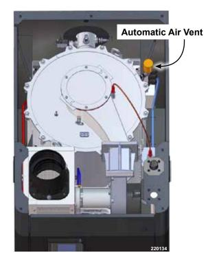
Figure 10 Automatic air vent cap and valve
