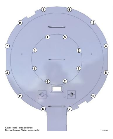
Figure 78 Tightening sequences – SVF 1000
