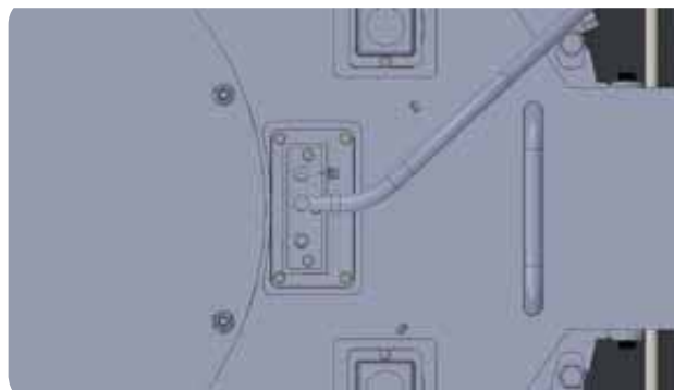
Figure 86 Correct orientation of ignition electrode / flame sense rod sight glass in down position.
