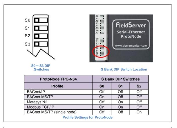
Figure 5: S Bank DIP Switches
