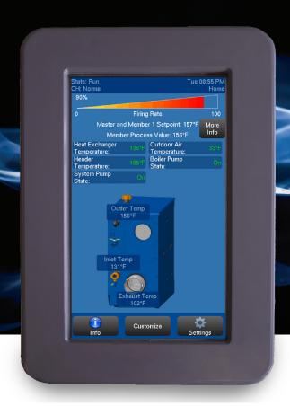
The Nuro Controller puts you in command of your heating system with easy installation, enhanced boiler diagnostics and remote monitoring capability.
