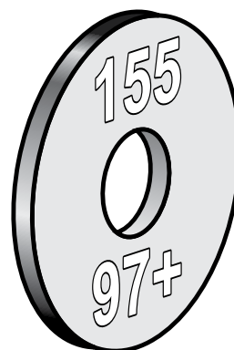
Figure 16 Propane gas orifice identification EVG 155
