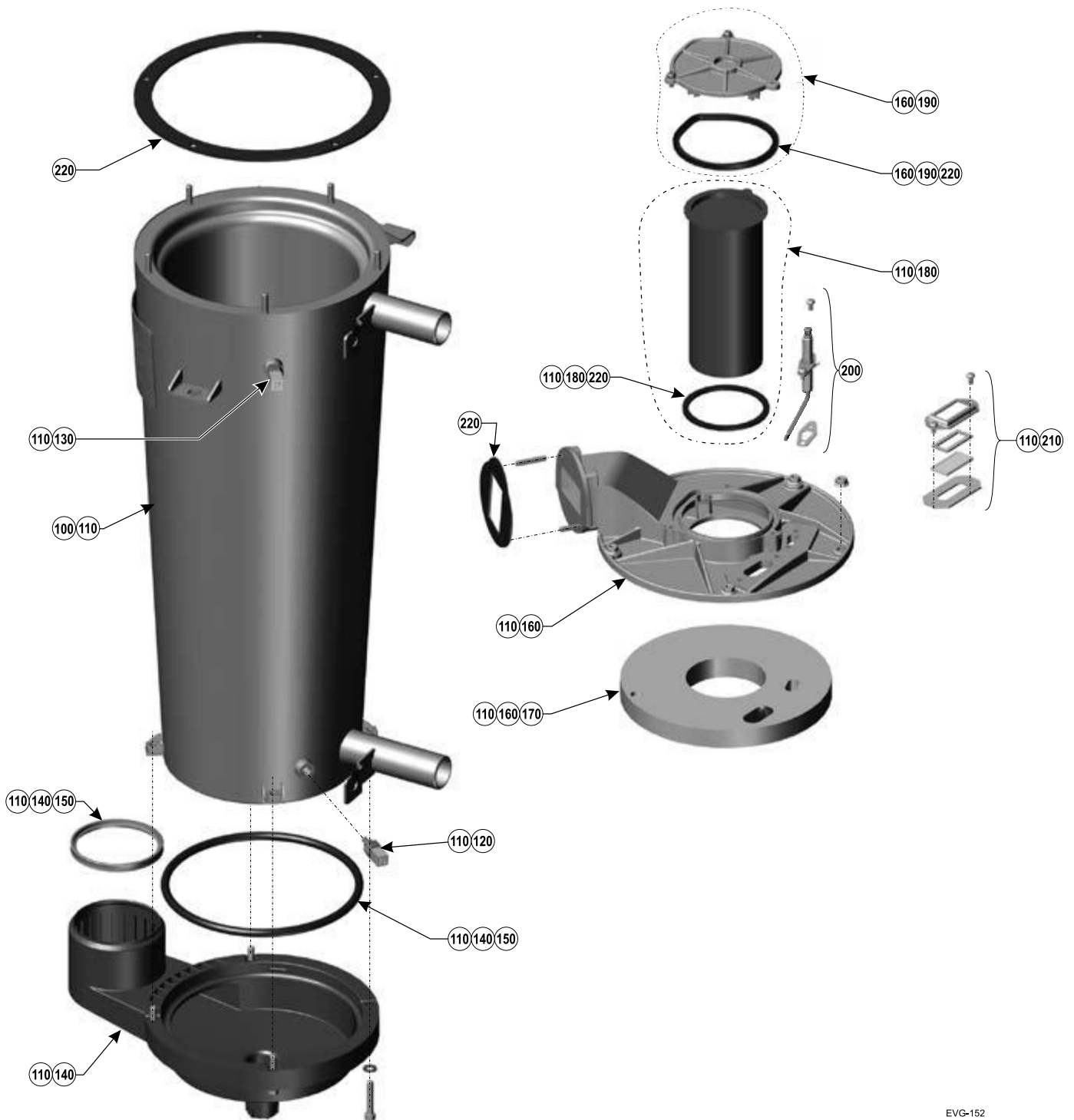
Figure 117 Heat exchanger assembly EVG 155 (see Figure 116, page 132 for part numbers)
