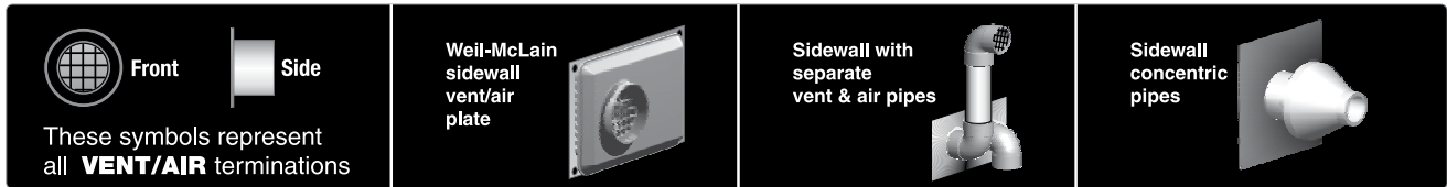
Figure 21 The vent termination must be located to meet all requirements below (also applies to vertical vent terminations). The minimum distance from adjacent public walkways, adjacent buildings, openable windows and building in the National Fuel Gas Code, ANSI Z223.1/NFPA 54 and/or the Natural Gas and Propane Installation Code, CAN/CSAB149.1. The vent termination clearances below are for U.S.A., for Canadian vent termination clearances please refer to the requirements of CAN/CSA B149.1 Natural Gas and Propane Installation Code. Consideration should be given to avoid possible damage caused by vent plumes and condensate when choosing a venting configuration and location. Maintain a minimum clearance of 4 ft. (1.22m) horizontally from, and in no case above or below, unless a 4 ft. (1.22m) horizontal distance is maintained, from electrical meters, gas meters, regulators, and relief equipment.
