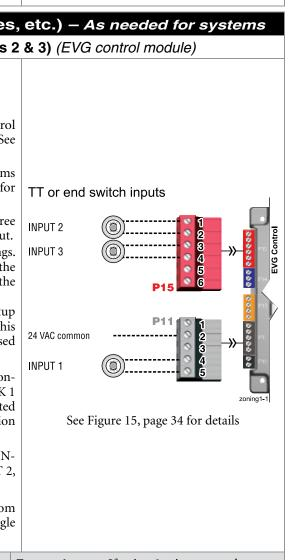
**Zone valves** — If using 3-wire zone valves, use relays to provide dry contacts to the Control thermostat connections. The zone valve end switches of 3-wire valves carry 24 VAC from the valve.
