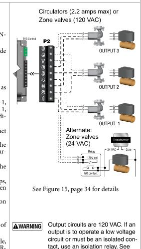
For circulators with higher amp ratings, install a circulator relay or starter. Connect only the 120 VAC coil to the Evergreen<sup>®</sup> circulator terminals.
