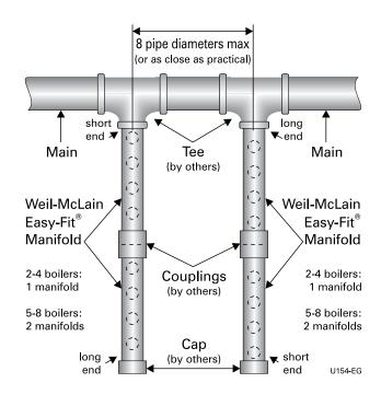
Figure 6 Double-sided EZ-Fit Header connection
