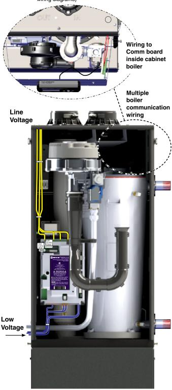
**WARNING** Installer MUST use a strain relief through jacket knockouts. Failure to do so can cause severe personal injury, death or substantial property damage.
