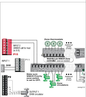
P15, P11, and P2 are terminal strips on the EVG control Relay **R1**, when used, is provided by installer
