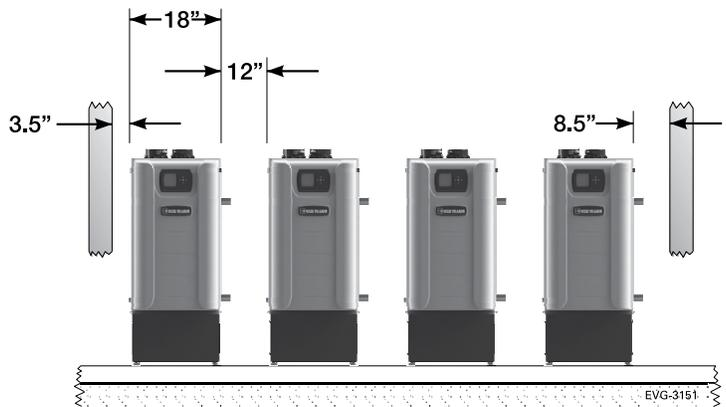
**Figure 4** Manifolded combustion air option
