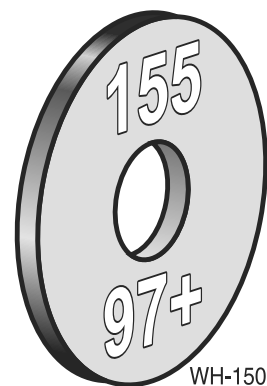
Figure 16 Propane gas orifice identification ECO 155
