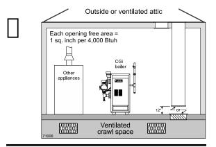
Figure 5 Air from outdoors — horizontal ducts
