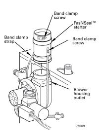
Figure 10 Saf-T Vent® vent starter
