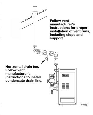
Figure 14 Direct exhaust sidewall venting
