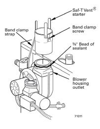
Figure 9 **Z-Vent II** vent starter
