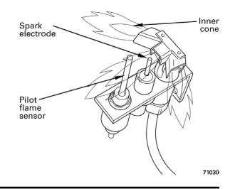
Figure 29 Typical main burner flame
