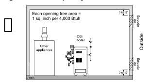
Figure 4 Air from outdoors — vertical ducts
