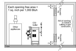
Figure 3 Air directly through outside wall
