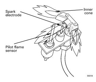
Figure 22 Typical main burner flame
