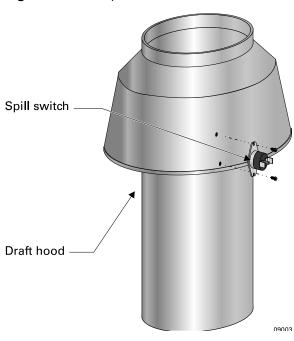
Figure 7 Spill switch with wire harness
