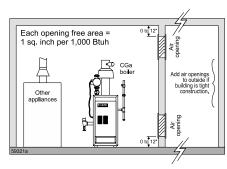
Figure 3 Air directly through outside wall
