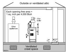
Figure 5 Air from outdoors — horizontal ducts
