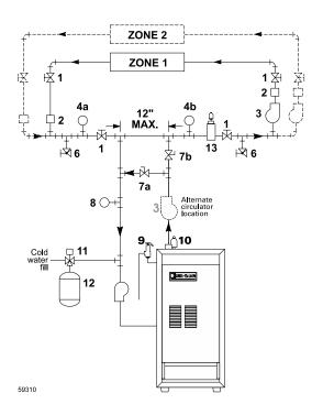
Figure 14 Primary/secondary piping Zoning with zone valves
