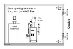
Figure 4 Air from outdoors — vertical ducts
