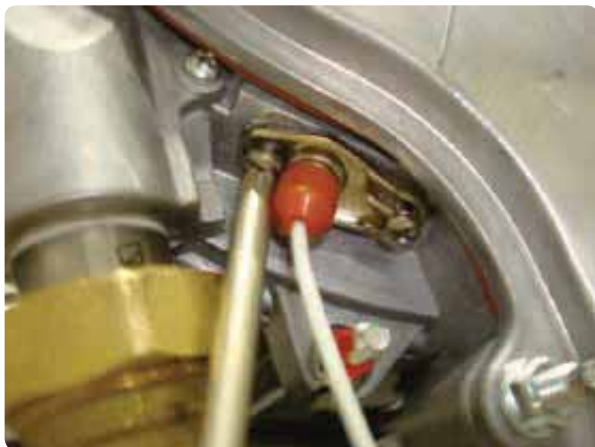
Figure 137 Removal of Ignition electrode
