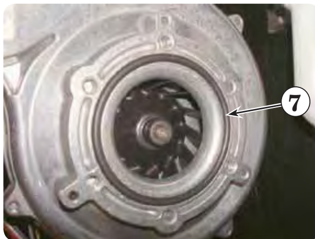
Figure 15 Insure "O" ring is in place
