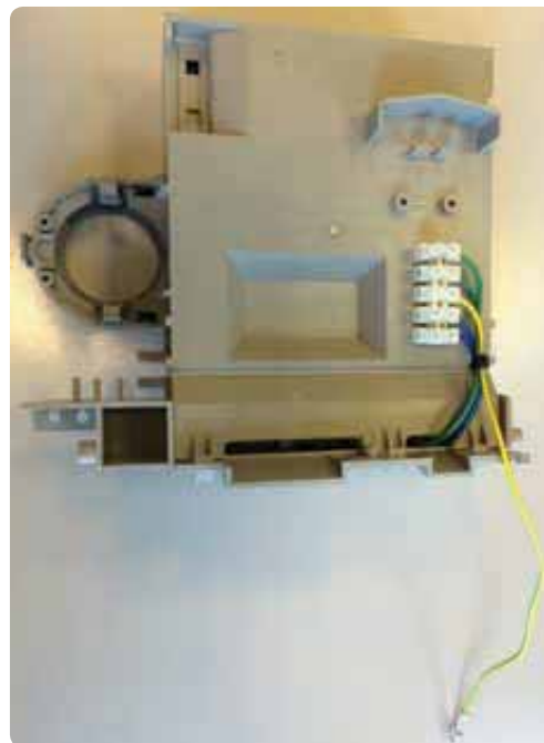
Figure 66 Circulator connectors (Heating Only boilers)
