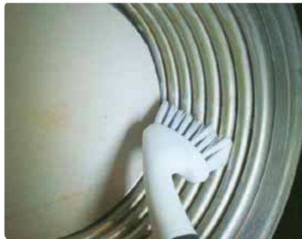
Figure 146 Cleaning the heat exchanger
