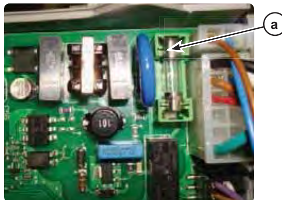
Figure 111 Thermostat-relay circuit fuse location
