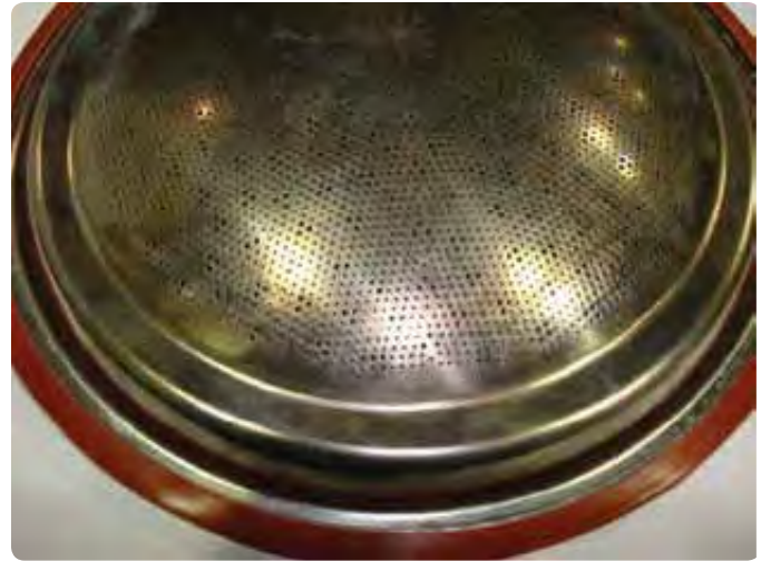
Figure 143 Inspecting exterior and cleaning the burner
