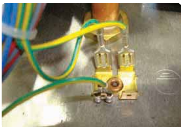
Figure 138 Ignition electrode grounding
