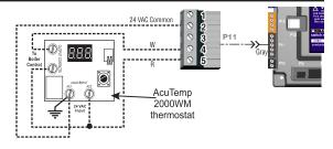
Wiring the control to GV90+ (1135-700), CGa (1135-05/606), CGi (1135-615), and the EG Water (1135-605) boiler controls
