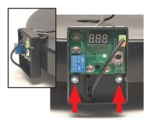
2 Route the sensor wire through the opening in the rear of the control
