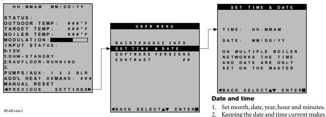
Figure 6 SlimFit boiler control display LOCKOUT SCREEN — screen turns red when boiler locks out — highlight and select MANUAL RESET to reset boiler as shown below.
