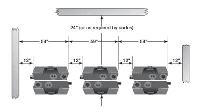
Figure 5 Manifolded combustion air option
