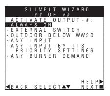
Use this screen to set when a SYSTEM PUMP/AUX output is activated. For detailed explanation, see Figure 34, page 57 and Figure 35, page 57.
