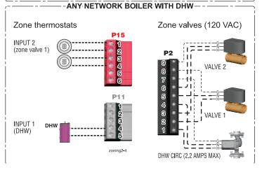
P15, P11, and P2 are terminal strips on the SlimFit control (See wiring at left for 24 VAC zone valves).
