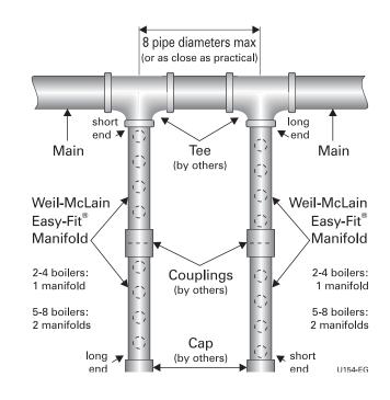
Figure 7 Double-sided EZ-Fit Header connection
