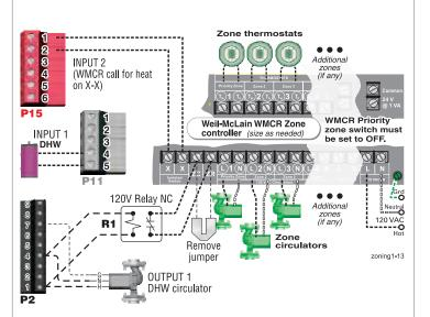
P15, P11, and P2 are terminal strips on the SlimFit control Relay **R1**, when used, is provided by installer
