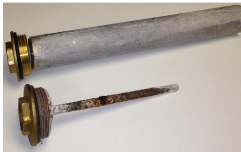
Depleted Sacrificial Anode
