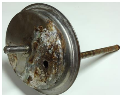
Leaking Corroded Drywell / Inspection Plate Due to Depleted Anode
