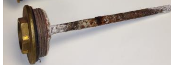
Depleted Sacrificial Anode
