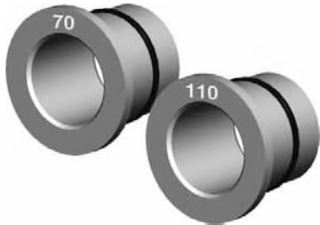
Figure 8 Propane gas orifice bushing identification WM97+70 on left (may be stamped 3.85) WM97+110 on right (may be stamped 4.45)
