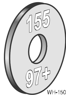
Figure 11 Propane gas orifice identification WM97+155
