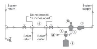
Alternate — Piping to closed-type expansion tank
