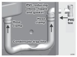
Figure 14 Condensate drain — Ultra-310
