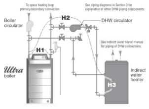
H1 = Head loss through boiler
