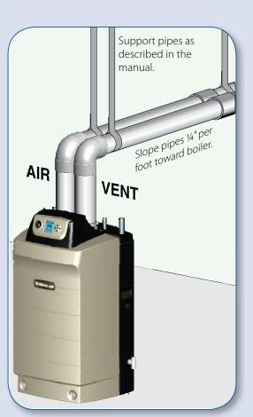
Slide the air inlet pipe and vent pipe into the boiler top openings. Just tighten the restraining rings — no messy sealants required. Reducers or adapters are required when the vent / air pipe O. D. is different from the boiler connection diameter (see below). All AL29-4C stainless pipe applications require adapters made by the vent pipe manufacturer. See the material checklist for items required.
