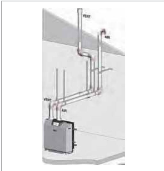
Figure 35 Maximum piping lengths for DIRECT VENT vertical termination
