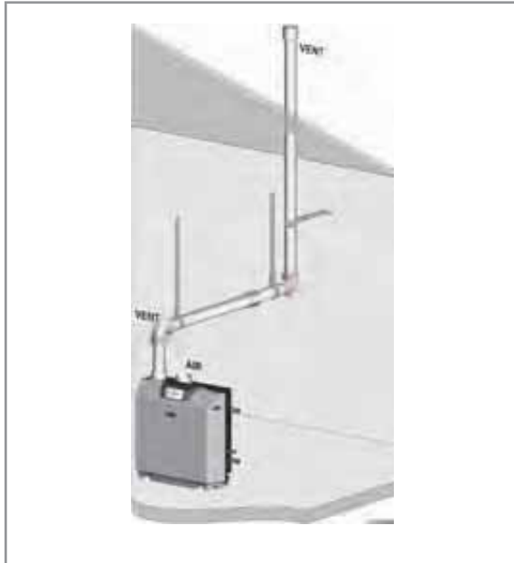
Figure 22 Maximum piping lengths for DIRECT EXHAUST vertical termination
