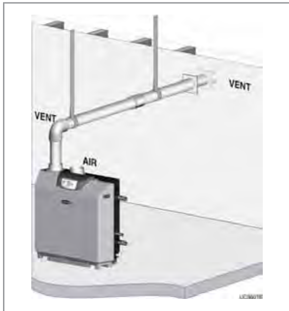
Figure 22 DIRECT EXHAUST — Sidewall termination
